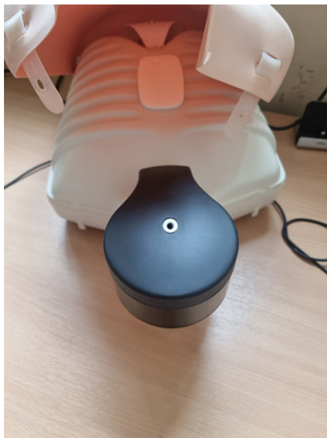
Figure 2: The ORSIM® black sensor box is placed over the head with an exit point towards the thorax.
